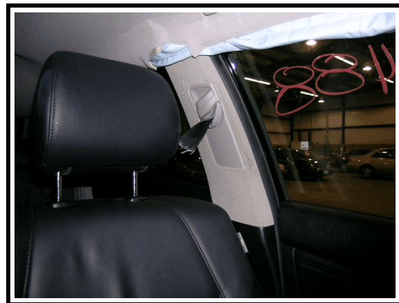
Figure 11. Driver's seat belt, cut by fire/rescue personnel.
