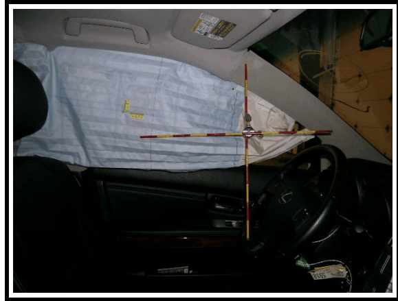
Figure 14. Possible occupant contact, Left side curtain air bag
