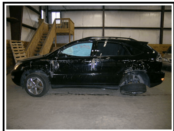
Figure 2. Left side rollover damage - 2005 Lexus RX330
