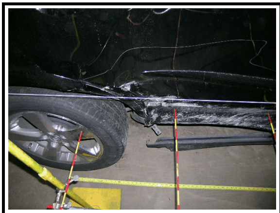
Figure 6. Case vehicle's right rear tire - Location of possible snag
