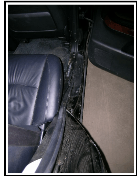
Figure 10. Second row, right sill intrusion
