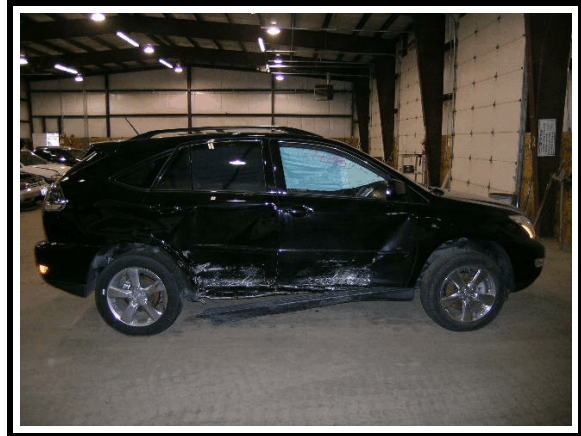
Figure 1. Right side impact damage - 2005 Lexus RX330
