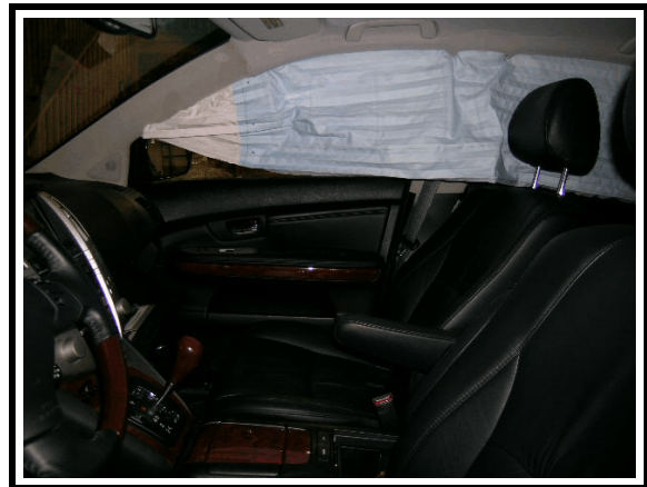
Figure 13. Right side curtain air bag, front row
