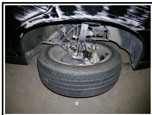
Figure 7. Damaged left rear axle - 2005 Lexus RX330
