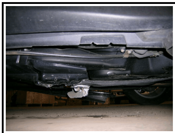
Figure 8. Damage to case vehicle's fuel tank and shield
