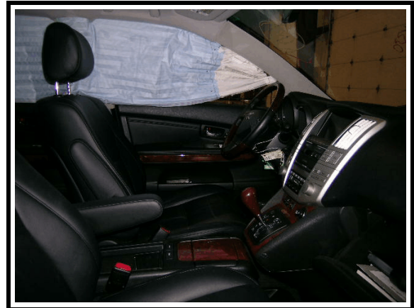
Figure 12. Left side curtain air bag, front row
