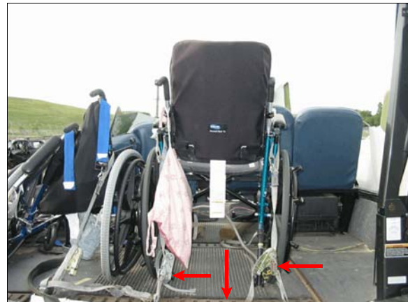
Figure 11: Right wheel chair, arrows show wheelchair securement straps secured to wheelchair and securement anchorage plate
