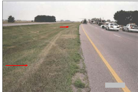
Figure 3: Police on-scene photo showing travel path of case vehicle in median, arrows show left side tire marks in grass
