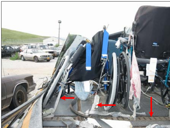
Figure 10: Deformation of left wheelchair, arrows show wheelchair securement straps secured to wheelchair and securement anchorage plate
