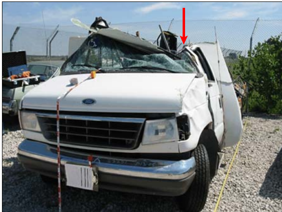
Figure 6: Damage to case vehicle's left roof and roof side rail from ground impact
