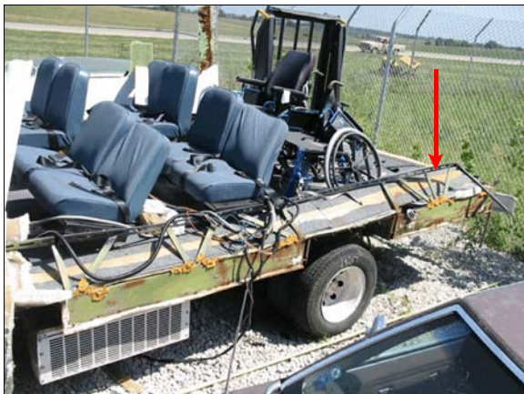
Figure 8: Left side view of passenger area, bus body was screwed to metal frame (arrow)
