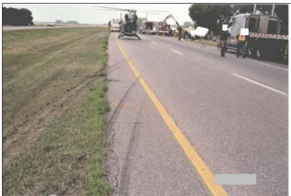
Figure 4: Case vehicle's yaw marks as it reenters roadway in clockwise rotation
