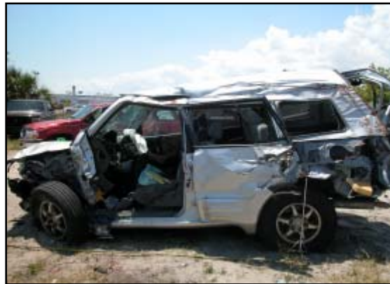
Figure 5. Left side damage to the Mitsubishi from the impact with the Lufkin trailer.
