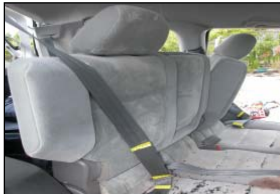
Figure 18. Loading evidence on right rear safety belt of the Montero.
