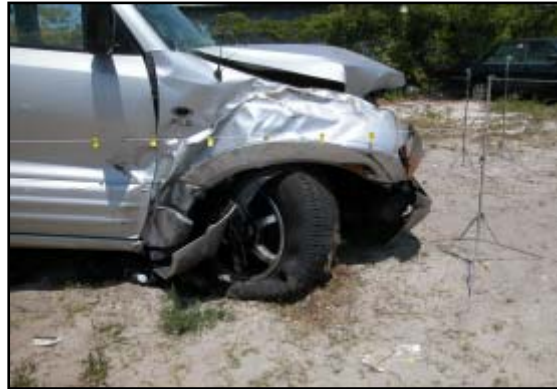
Figure 7. Right side damage to the Montero from the secondary impact with the Ford
