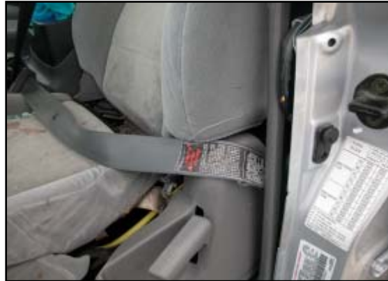
Figure 16. Mitsubishi's driver's lap belt with deployed energy management loop.
