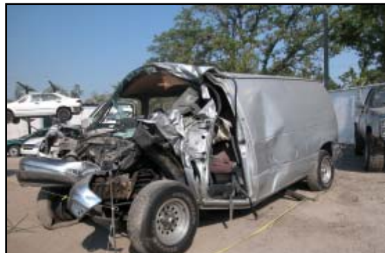
Figure 13. Ford’s windshield header damage and crush profile.
