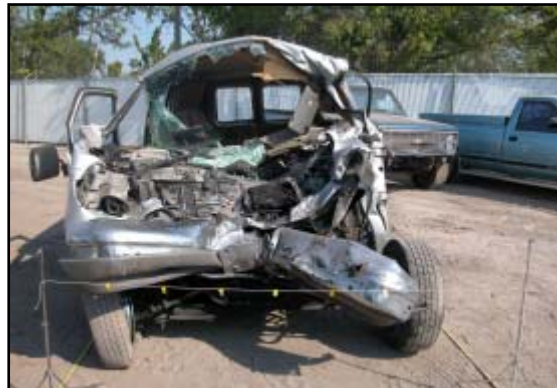
Figure 12. Frontal damage to the Ford from the impact with the Mitsubishi.
