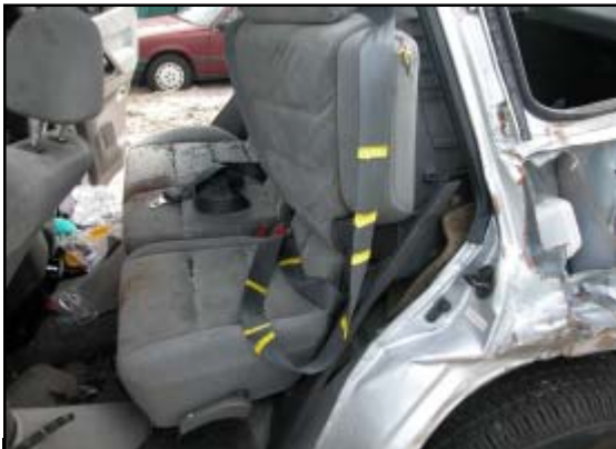
Figure 17. Loading evidence on left rear safety belt of the Montero.
