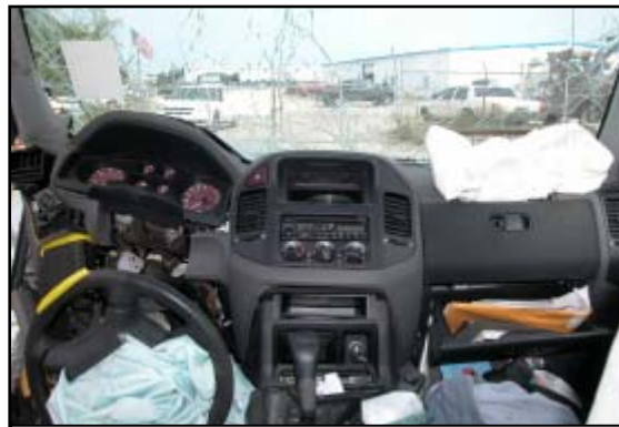
Figure 8. Interior damage to the first row of the Montero.
