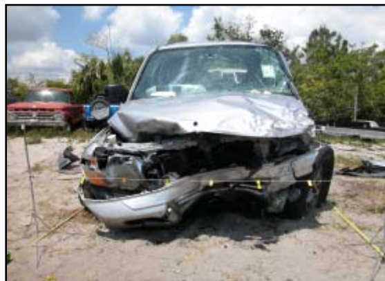
Figure 6. Frontal damage to the Mitsubishi from the impact with the Ford.
