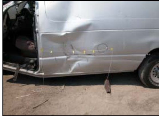
Figure 14. Left side damage to the Ford from the impact with the Mitsubishi's right rear tire.
