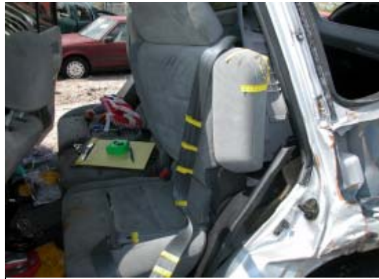
Figure 11. Forward deformation of the second row seatbacks of the Mitsubishi and left seatback contact from the Lufkin trailer.
