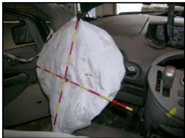
Figure 18: View of the deployed air bags.
