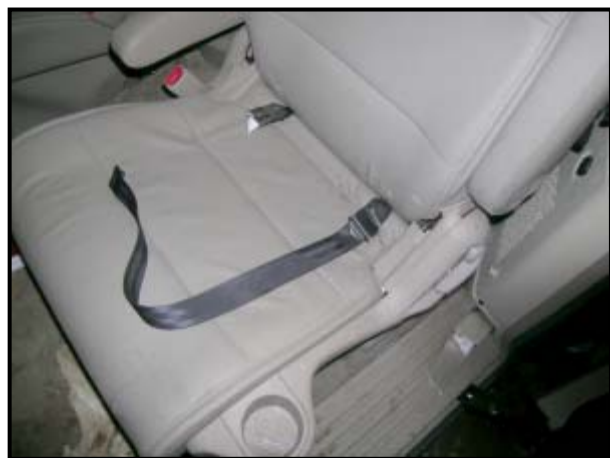
Figure 16: Cut seat belt of the Row 2 left seat.
