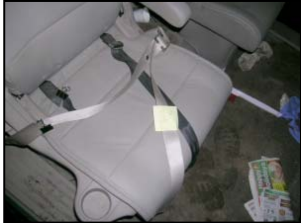
Figure 17: Second row right seat cut vehicle seat belt and cut LATCH webbing.
