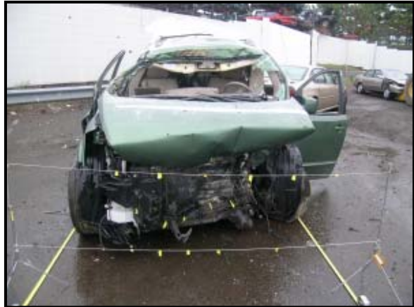
Figure 7: Nissan frontal damage.
