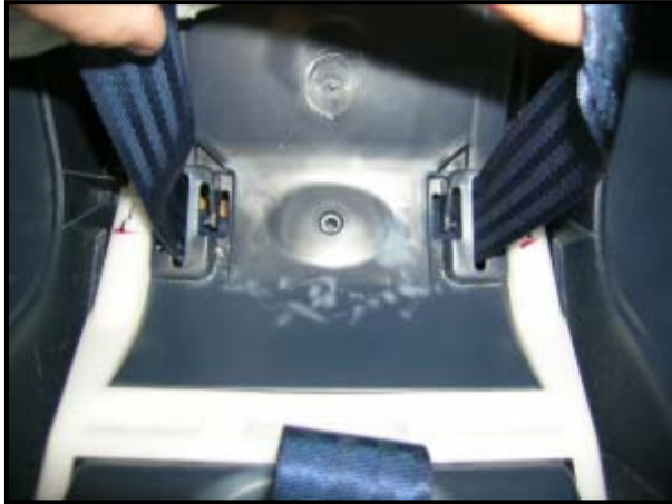
Figure 21: Stress marks in the bucket of the left CSS shell.
