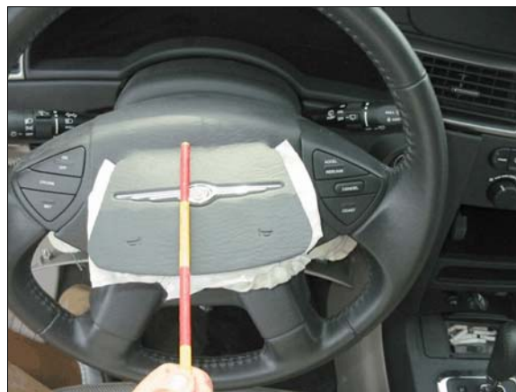
Figure 9: Driver's air bag module cover flap
