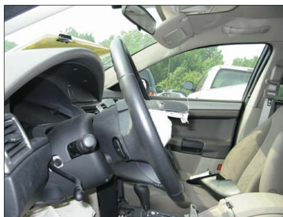
Figure 8: Left side view of steering wheel and steering column showing lack of deformation
