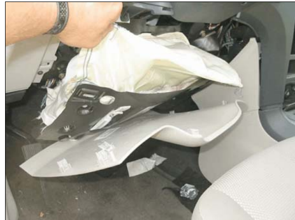
Figure 12: Case vehicle driver's inflatable knee blocker
