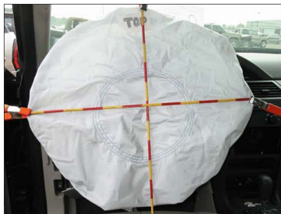
Figure 11: Case vehicle driver's air bag
