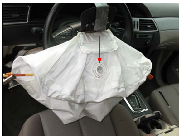
Figure 10: Case vehicle driver's air bag vent port
