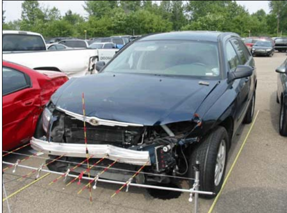
Figure 4: Overview of damage to front of case vehicle from impact with the Sebring, each increment on the rods is 5 cm (2 in)
