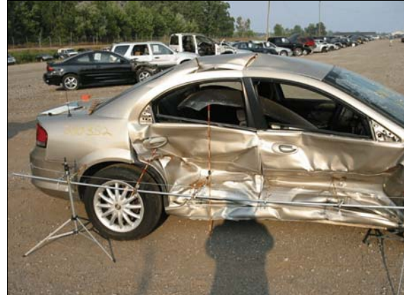
Figure 5: Damage to right side of the Sebring from impact with the case vehicle
