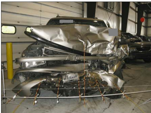
Figure 3: Damage to front of case vehicle from impact with front of Silverado, each increment on rods is 5 cm (2 in)
