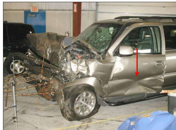
Figure 4: Overview of damage to left front door from impact with front right bumper corner of Silverado
