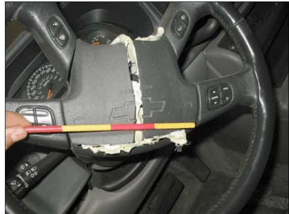
Figure 9: Driver's air bag module flaps, steering wheel is rotated counterclockwise approximately 140 degrees
