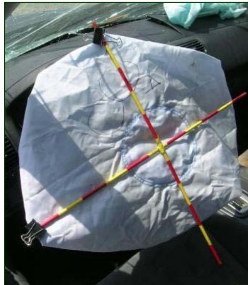
Figure 8. Circled areas of suspected transfers on the driver's air bag.
