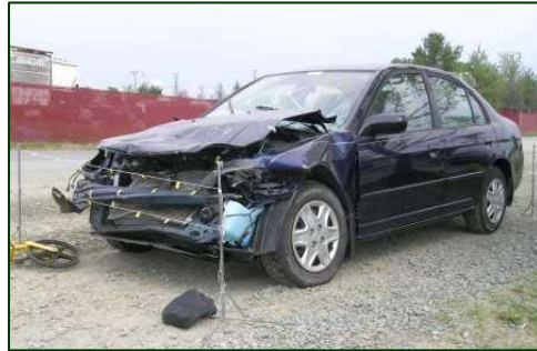
Figure 1. Frontal damage to the 2003 Honda Civic.
