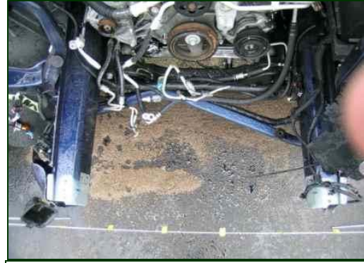
Figure 5. Overhead view of the crush depth to the lower radiator support.
