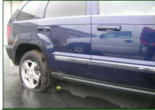
Figure 7. Right rear impact damage.
