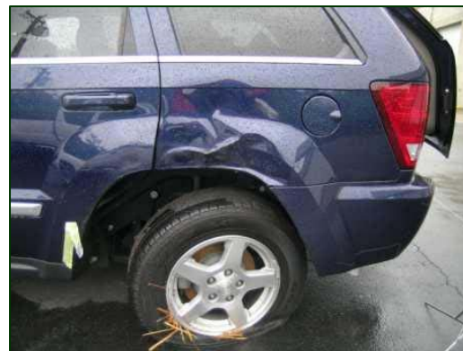
Figure 6. Left rear impact damage.
