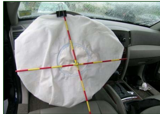
Figure 8. Deployed front left air bag.
