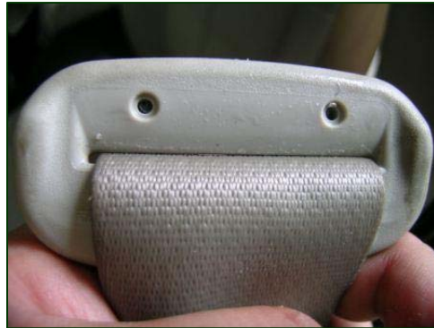
Figure 10. Frictional abrasion of the driver's latch plate.
