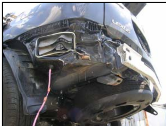
Figure 5: Left rear damage to the Lexus.
