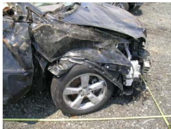
Figure 6: Impact damage to the right front fender.
