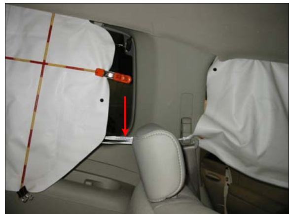
Figure 15: Overview of tether (arrow) between the back left side curtain air bag and the second seat left side curtain air bag
