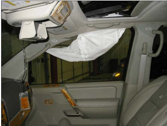
Figure 16: Overview of front right passenger's side curtain air bag, it did not break through the headliner at the "B"-pillar during deployment
