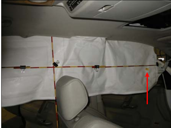
Figure 12: Case vehicle's driver and second seat left side curtain air bag, arrow shows location of a small scuff mark on the air bag
