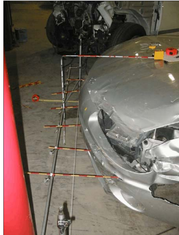
Figure 6: Damage to front of Oldsmobile from impact with the Geo, each increment on rods is 5 cm (2 in)
