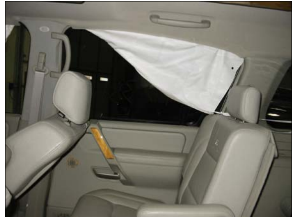
Figure 17: Overview of front right passenger's/second seat right side curtain air bag, it did not break through the headliner at the "B"-pillar during deployment
