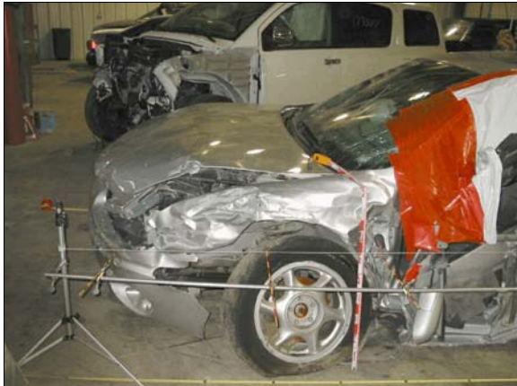
Figure 5: Damage to Oldsmobile’s left fender and left front door from impact with the case vehicle, each black mark on tape measure is 0.31 meter (1 foot)
