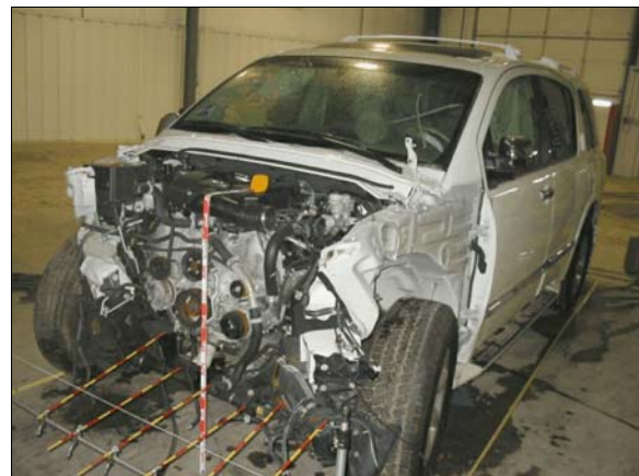
Figure 4: Overview of damage to front of case vehicle, damaged components had been removed and disposed, each increments on tape measure is tenth of meter
