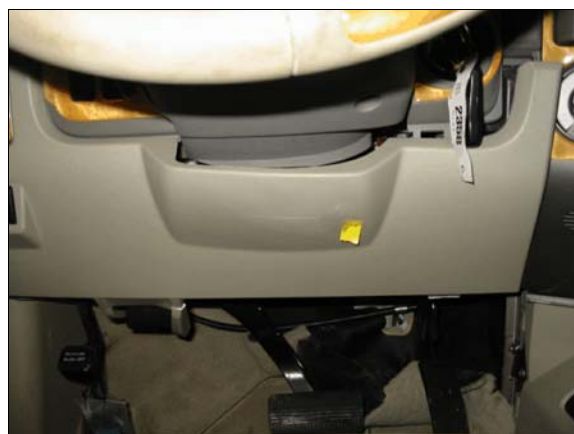
Figure 19: Driver's knee bolster is displaced, yellow tape shows scuff from driver knee contact
