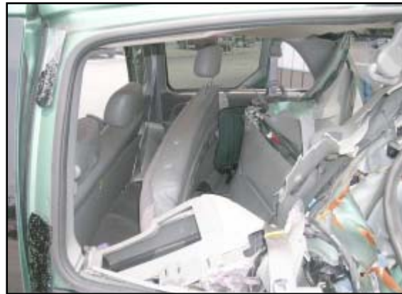
Figure 7. Third row intrusion and displaced third row bench seat.
