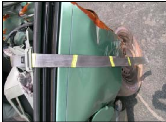
Figure 8. Third row left safety belt transfers and loading evidence.
