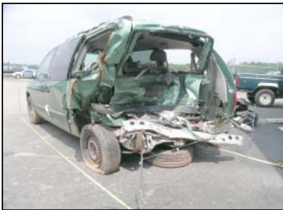
Figure 3. Overall view of the rear damage.
