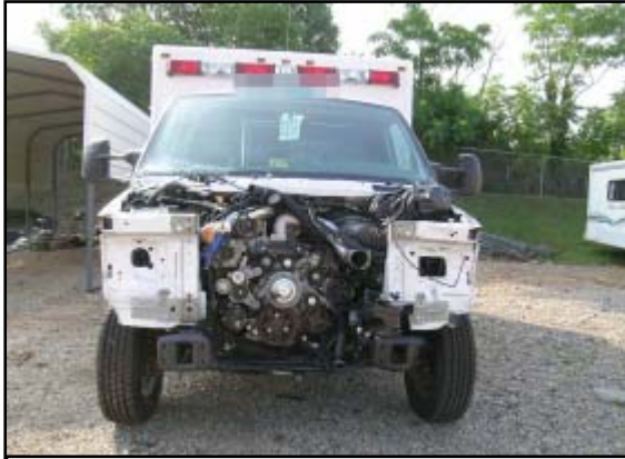
Figure 5. Dismantled frontal structure
