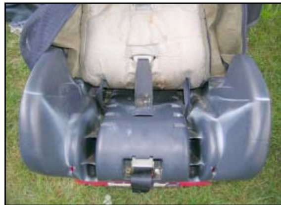
Figure 10. Stress marks on the seat cushion aspect.
