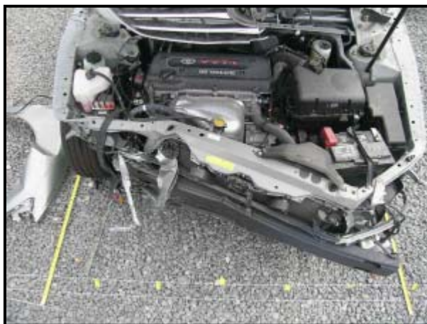
Figure 5: Overhead view of the Camry depicting the extent of crush.
