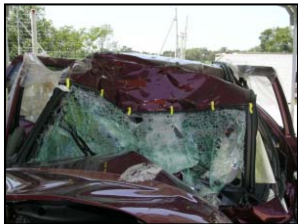
Figure 8: Front view of the damage header.
