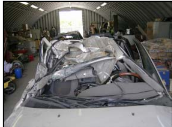
Figure 11: View of the deformed roof.
