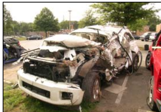
Figure 6. Overall view of the frontal and left side damage.
