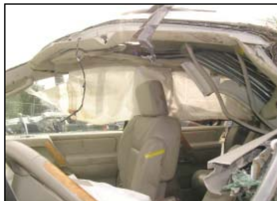
Figure 8. Deployed right side curtain air bag.
