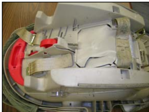
Figure 11: View of the fractured shell.
