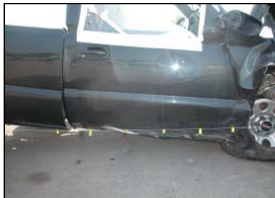
Figure 6. Right side damage from the tree stump impact.
