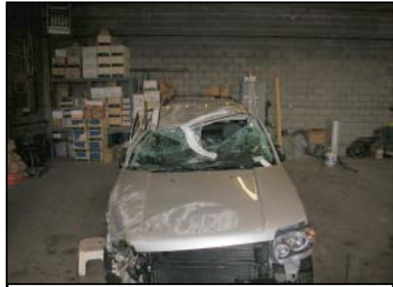
Figure 7. Roof crush profile.
