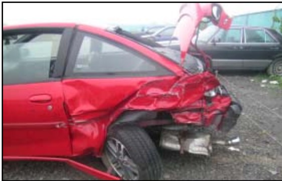
Figure 8. Direct contact damage on the left side.
