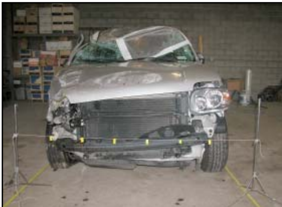
Figure 5. Frontal damage from the impact with Chevrolet.
