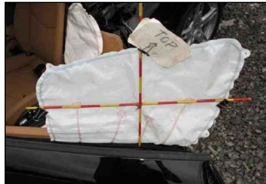
Figure 12 - Door mounted head protection air bag.
