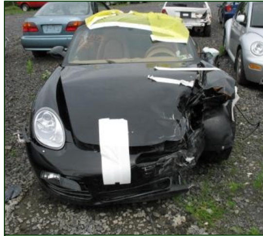
Figure 1. Front left damage to the Porsche Boxster.
