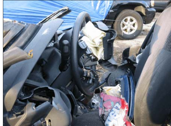
Figure 10: Left side overview of damage to case vehicle's steering wheel and steering column, air bag module torn open
