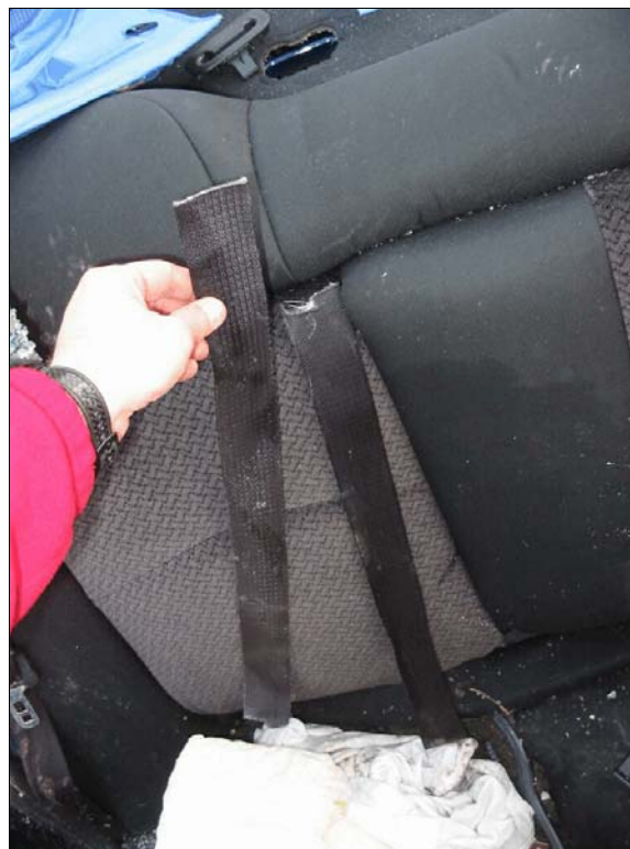
Figure 16: Case vehicle's back center safety belt cut by rescue personnel
