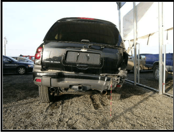
Figure 4. Back right damage - 2005 Chevrolet Trailblazer
