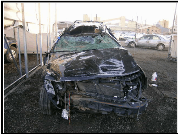
Figure 6. Rollover damage - 2005 Chevrolet Trailblazer
