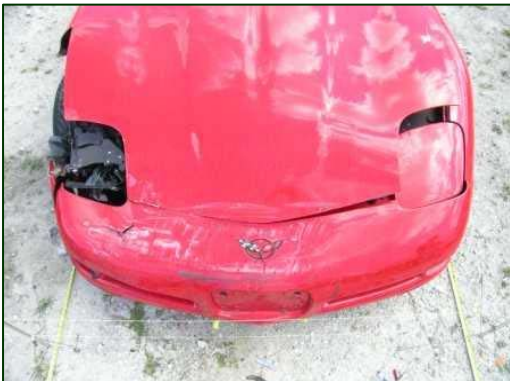
Figure 4. Overhead view of the direct contact damage.
