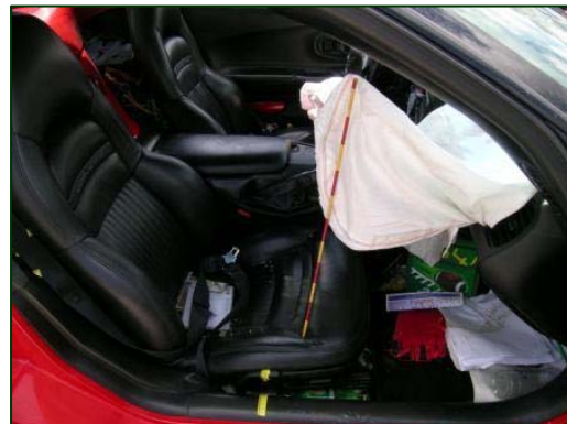
Figure 13. Lateral view of the child's trajectory and the deployment path of the front right air bag.
