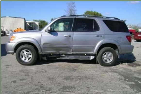
Figure 7. Left side damage to the Toyota Sequoia.
