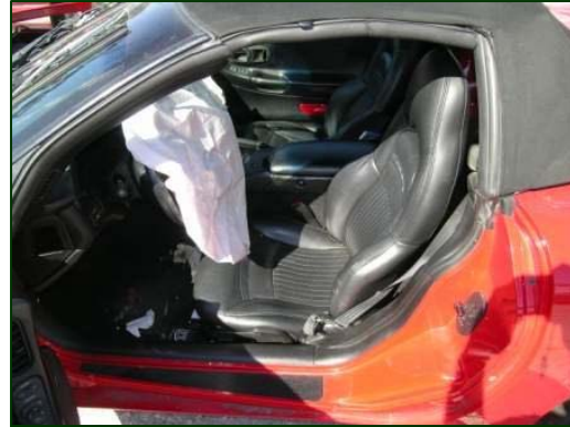
Figure 12. Lateral view of the driver’s position and the deployed front left air bag.
