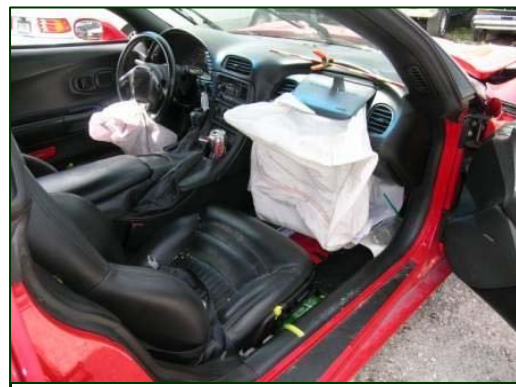
Figure 10. Deployed redesigned frontal air bags.
