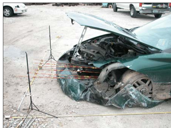
Figure 6: Left side view of crush to front of case vehicle from culvert impact, measurements were taken to the bumper bar, plastic bumper fascia was separated from the bumper bar
