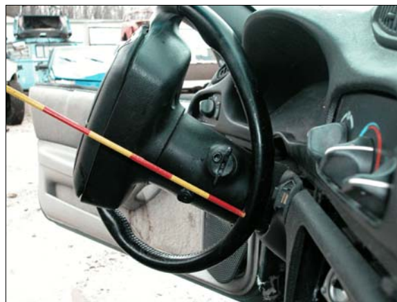
Figure 8: Right side view of deformation of steering wheel
