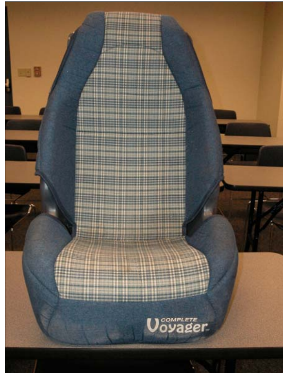
Figure 10: Front view of back right passenger's high back belt positioning booster seat
