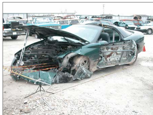
Figure 5: Front left overview of damage to case vehicle
