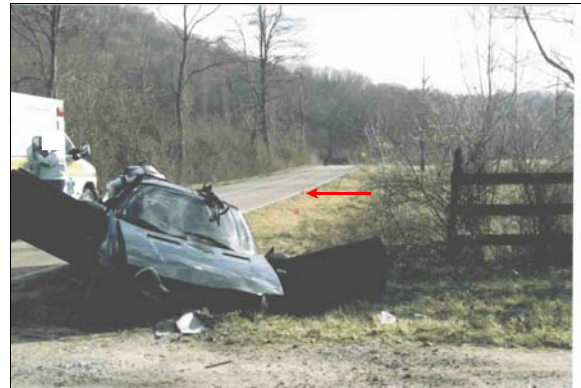
Figure 4: Police on-scene photo showing rest position of case vehicle, red flags show case vehicle's left side tire mark in grass (arrow)
