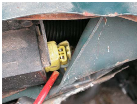
Figure 9: Front crash sensor receptacle was found broken and sensor was unplugged, plug moved to right for photo
