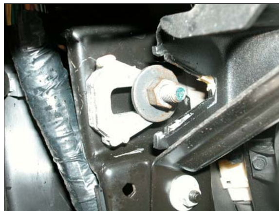
Figure 15: Separation of case vehicle’s right shear capsule and shear plate due to steering column loading by driver, left seat capsule also separated
