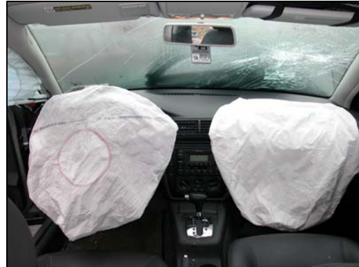
Figure 6 - Frontal air bag deployment - 2005 Volkswagen Passat.
