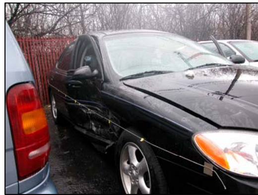
Figure 5 - Right side damage 2000 Ford Taurus.
