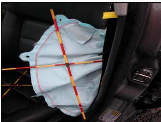
Figure 7 - Deployed side impact seat bag - 2005 Volkswagen Passat.
