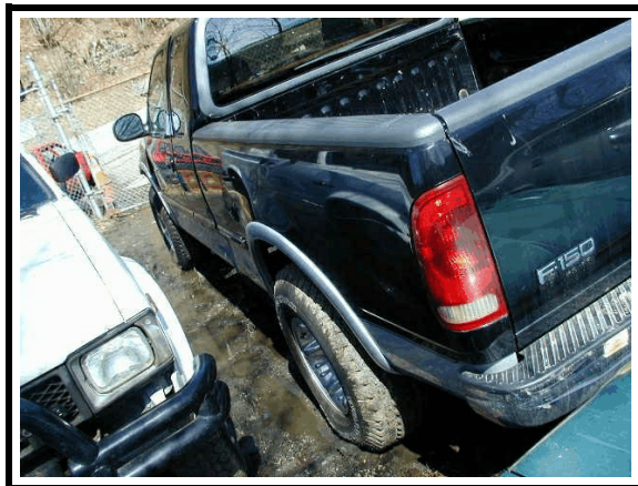
Figure 3. Left rear tire under-inflated at inspection
