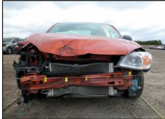
Figure 6. Frontal view of the crush to the Cobalt.
