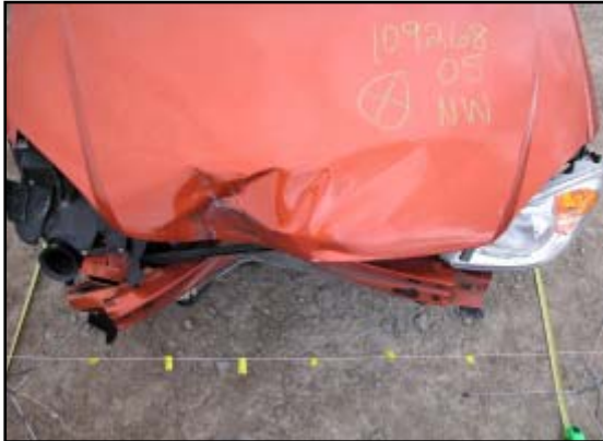
Figure 5. Overhead view of the frontal damage.
