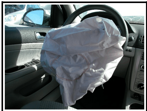
Figure 6. Driver's deployed air bag
