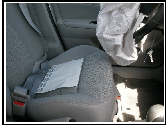
Figure 8. Driver’s seat belt (Retractor pretensioner actuated)
