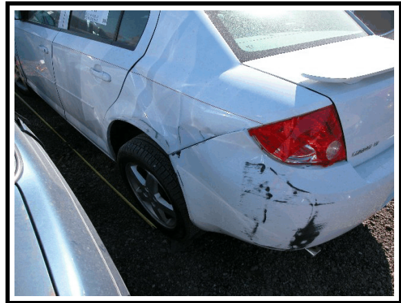
Figure 5. Left rear damage - 2006 Chevrolet Cobalt
