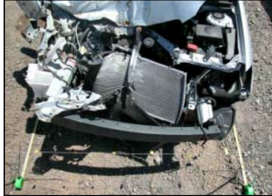
Figure 5. Overhead view of the residual crush to the frontal structure.
