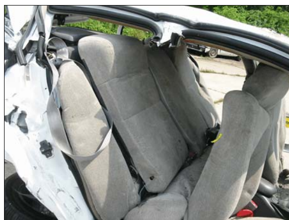
Figure 10: Intrusion of case vehicle's back seat, view from passenger side
