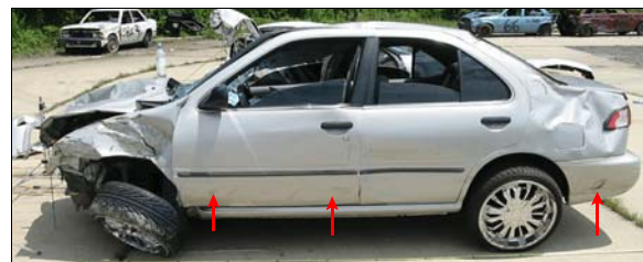
Figure 2: Damage to left side of Nissan from sideswiping right side of Chevrolet, arrows show tire marks from Chevrolet's left front wheel, damage on upper quarter panel is from rollover
