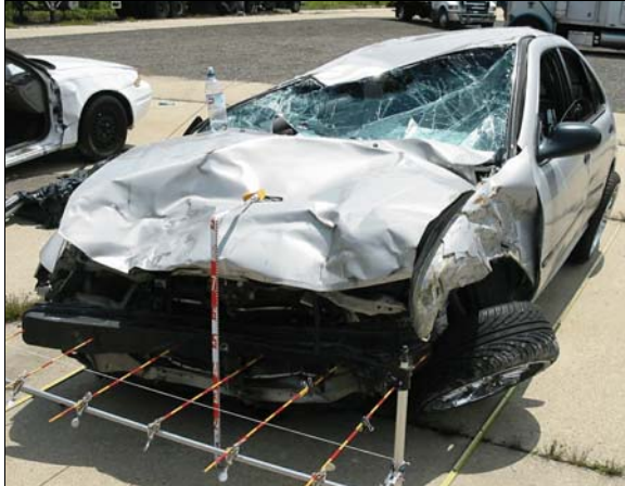
Figure 4: Damage to front of Nissan from impact with back of case vehicle, increments on vertical scale are tenths of meter, each increment on rods is 5 cm (2 in)
