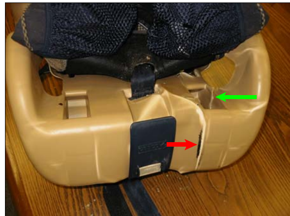
Figure 14: Damage to back center passenger's child safety seat, red arrow show fabric transfer on front of seat cushion, green arrow shows fractures in plastic
