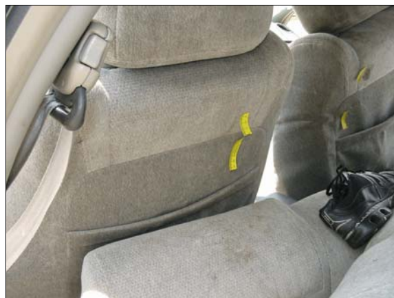
Figure 18: Occupant contact marks on driver's seat back
