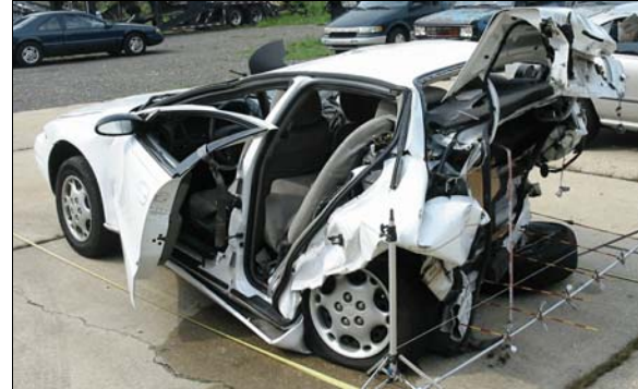
Figure 5: Damage to back of case vehicle from impact with front of Nissan, baseline set 100 cm (39.4 in) short of overall length due to insufficient length of measurement rods to capture totality of crush
