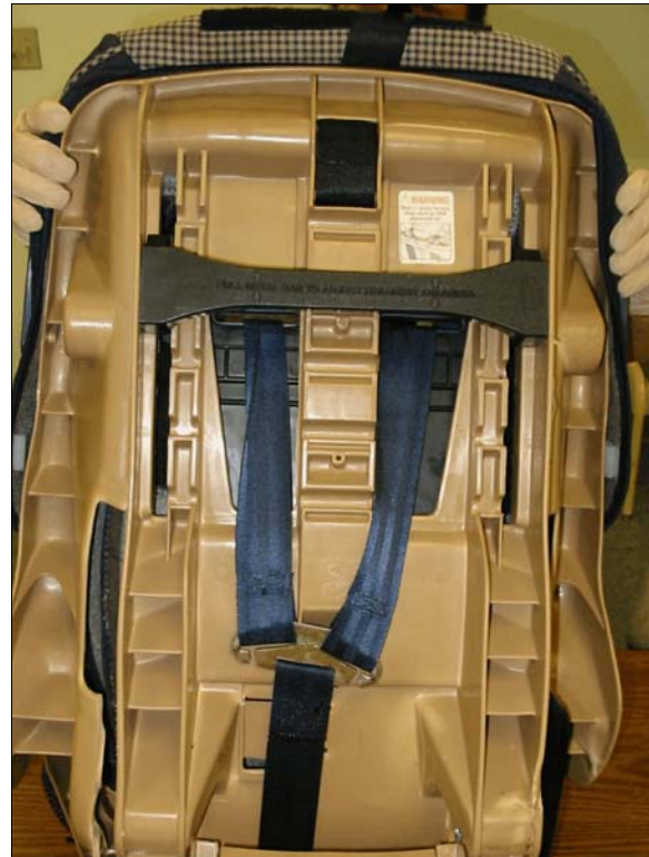
Figure 13: Back of back center passenger's child safety seat showing harness strap slots and harness adjuster mechanism
