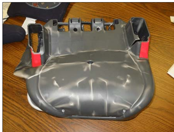
Figure 15: Deformation to case vehicle's back left passenger's booster seat
