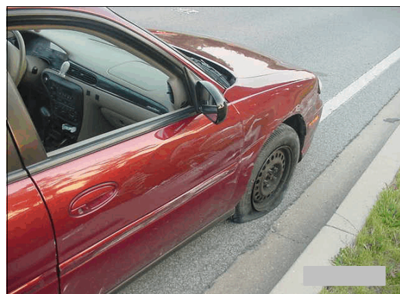
Figure 3: Police photo showing sideswipe damage to right side of Chevrolet from impact with left side of Nissan
