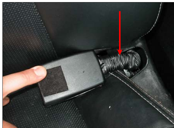
Figure 13: Case vehicle's front right passenger safety belt buckle, arrow shows retracted buckle stalk due to activation of pretensioner
