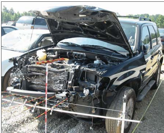
Figure 4: Damage to front of case vehicle from impact with the Saturn, increments on vertical scale in tenths of meter
