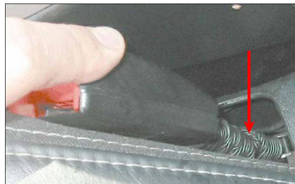
Figure 12: Case vehicle driver's safety belt buckle stalk, arrow shows retracted buckle stalk due to activation of the pretensioner
