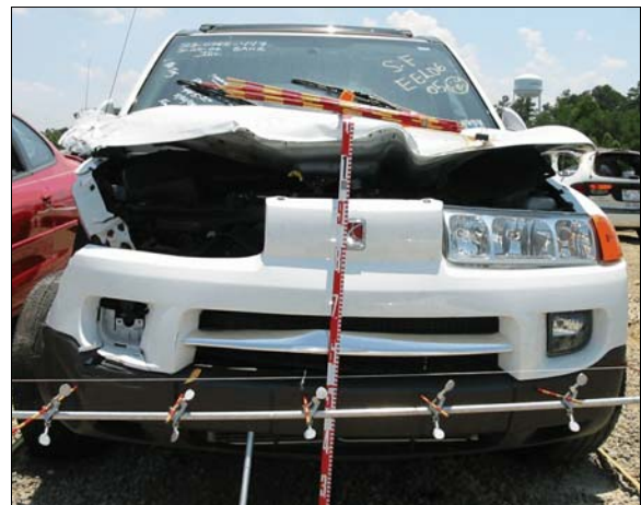
Figure 5: Damage to Saturn's front right corner from impact with case vehicle, deformations at middle of hood are not crash related, hood was pried open
