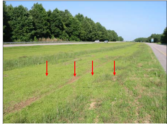
Figure 3: Case vehicle's yaw mark furrows in median, arrows show yaw marks, marks are from left to right: left front, right front, left rear and right rear
