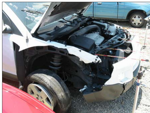
Figure 14: Right side view of damage to Saturn’s front bumper, right fender and right front wheel due to impact with front of case vehicle
