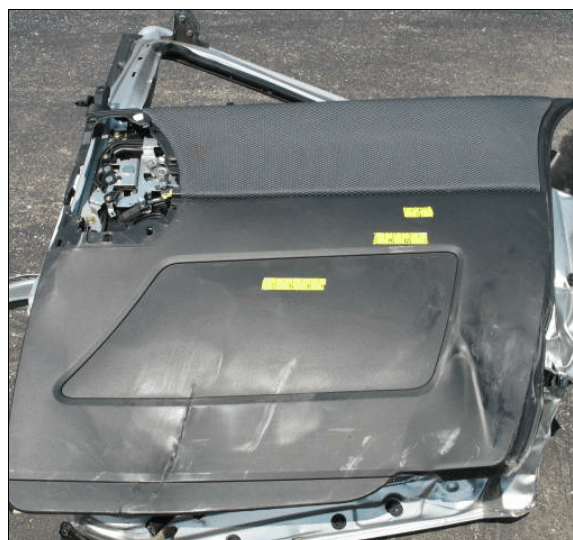
Figure 27: Overview of right rear door, yellow tape shows likely occupant contact marks
