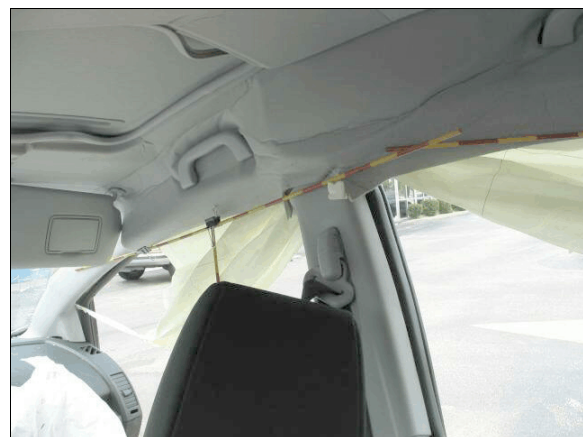
Figure 14: Overview of right side curtain air bag, it did not break out of the headliner at the "B"-pillar, each increment on rods is 5 cm (2 in)
