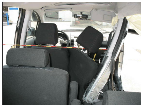
Figure 9: Overview of right "B"-pillar intrusion
