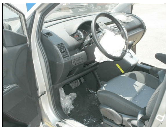
Figure 11: Overview of steering wheel and instrument panel, yellow tape shows occupant contact mark on center console
