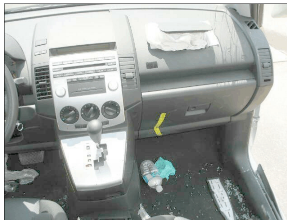
Figure 12: Overview of center and front right instrument panel, yellow tape shows occupant contact mark on glove box door and lower instrument panel
