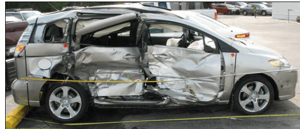
Figure 6: Damage to case vehicle's right side due to impact with front of Ford, right side doors placed back on vehicle in approximate crushed position
