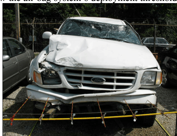
Figure 28: Damage to front of Ford from impact with the right side of the case vehicle and damage to the roof from the rollover
