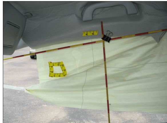
Figure 17: Right side curtain air bag adjacent to front right seat position, yellow tape on air bag shows location of possible skin transfer from front right occupant
