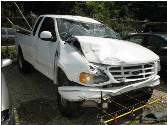
Figure 5: Right front view of damage to front of Ford from impact with the right side of the case vehicle and rollover damage to roof and hood.
