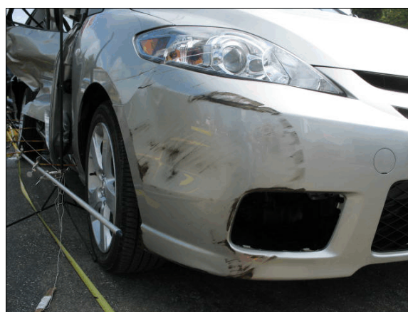
Figure 10: Damage to right front corner of case vehicle due to secondary impact with V2's right front wheel
