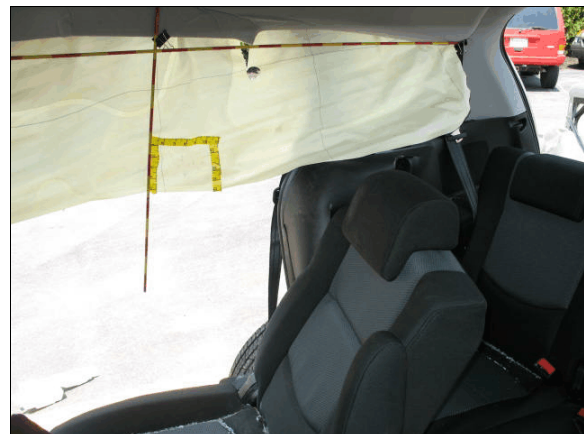
Figure 18: Overview of right side curtain air bag adjacent to second seat right passenger, yellow tape shows location of possible occupant contact mark
