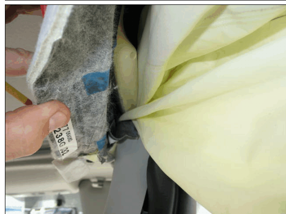
Figure 15: Close view of air bag bunched up behind headliner at right "B"-pillar, view is from back of "B"-pillar
