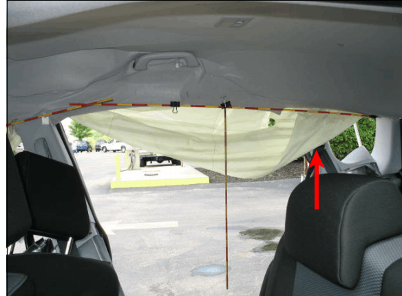
Figure 16: Overview of side curtain air bag adjacent to second seat right position, air bag did not break out of headliner at “B”-pillar and did not completely unfold at “C”-pillar (arrow)
