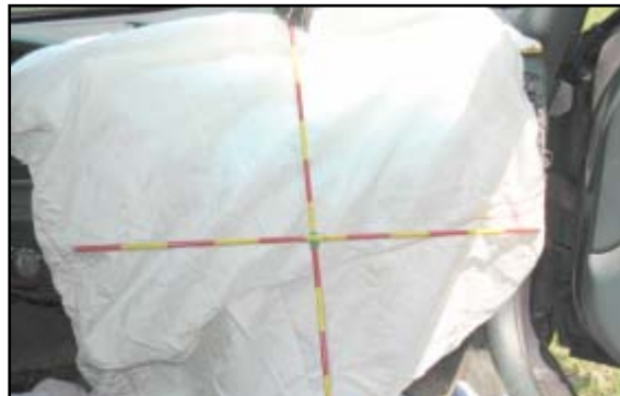
Figure 10. Deployed front right air bag.
