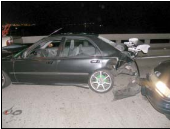
Figure 8. Resultant damage to the Honda.
