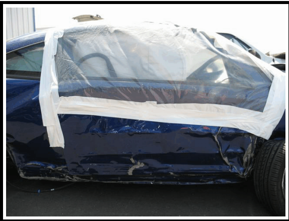
Figure 16. Right side tree impact damage
