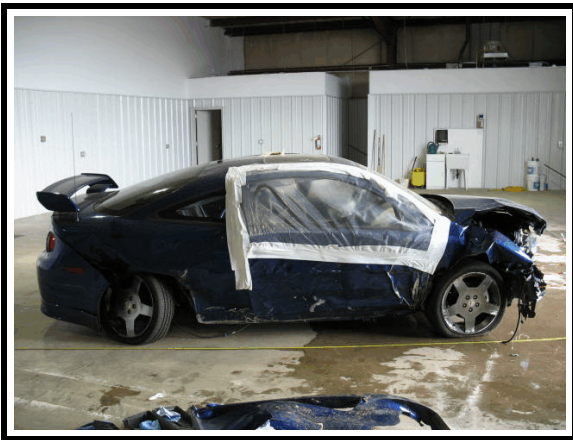
Figure 14. Right side damage
