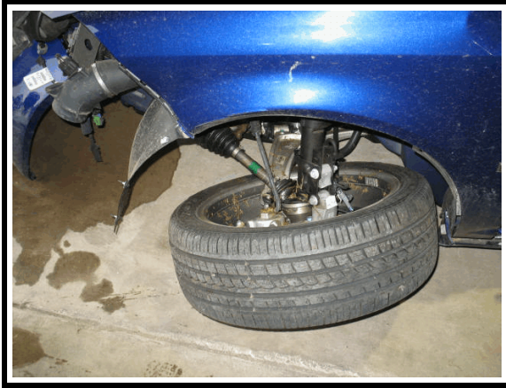
Figure 18. LF tire/axle damage
