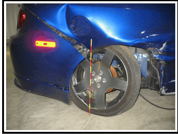
Figure 19. Damage to RR tire
