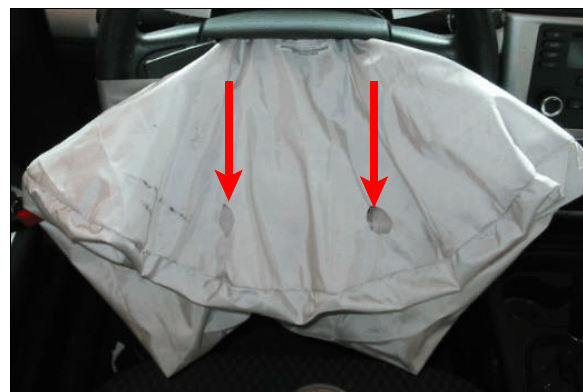
Figure 16: Arrows show case vehicle driver's air bag vent ports
