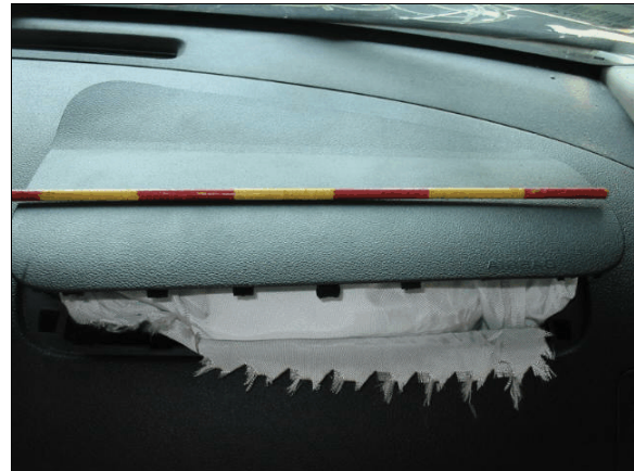
Figure 17: Case vehicle's front right passenger air bag module cover flap
