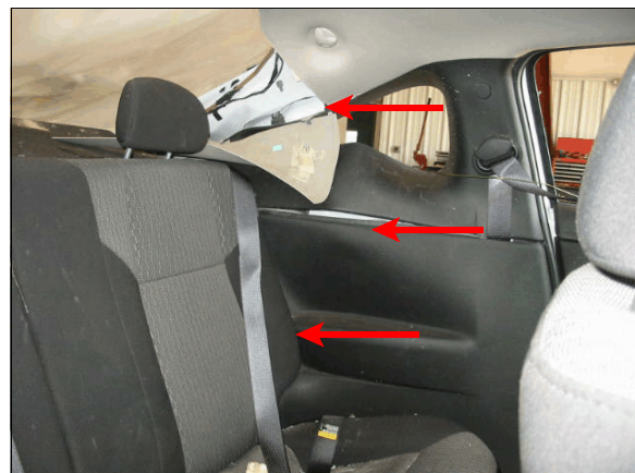
Figure 12: Overview of case vehicle's back left seat position, arrows show intrusion
