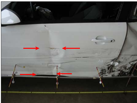
Figure 8: Guard rail post direct damage (arrows) to case vehicle's left front door and sideswipe damage from impact with Mercury
