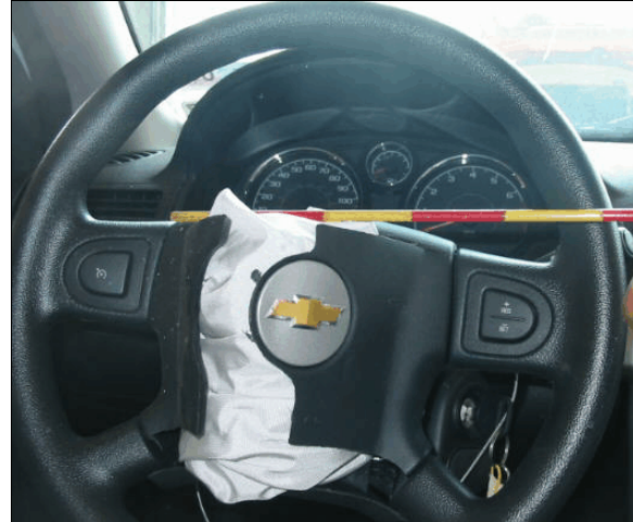
Figure 14: Case vehicle driver's air bag module cover flaps
