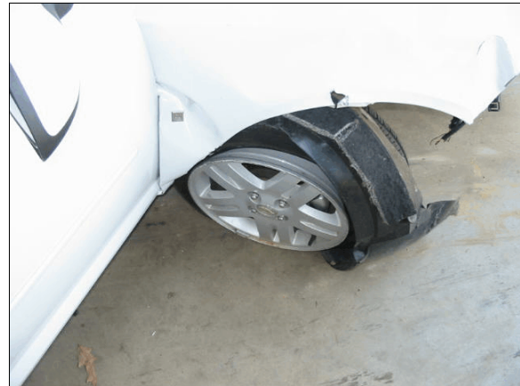
Figure 7: Displacement of right front wheel from snagging guardrail
