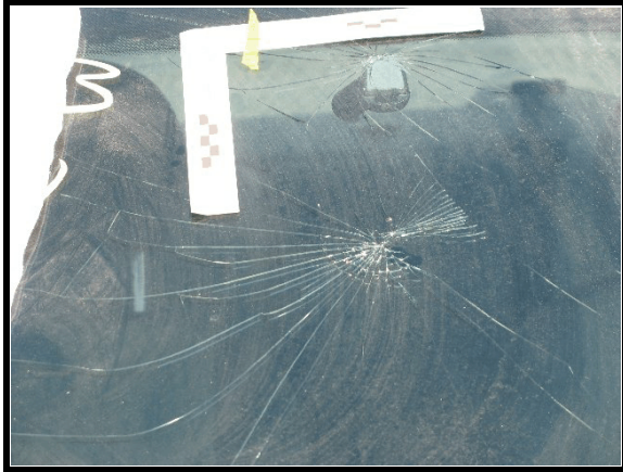
Figure 8. Damage to windshield from mirror
