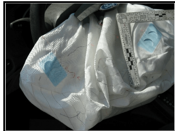
Figure 14. Vent ports, top module cover, driver’s air bag
