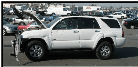
Figure 6. Left side rollover damage, 2006 Toyota 4Runner
