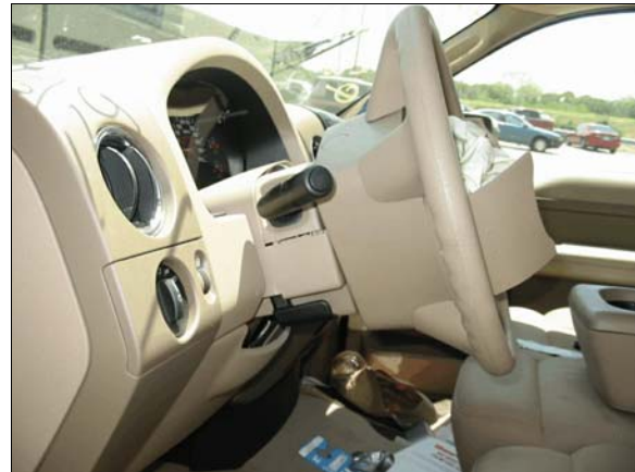
Figure 10: Left side view of case vehicle's steering assembly showing displacement of column cover
