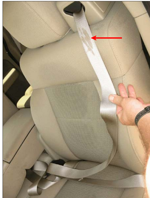
Figure 13: Case vehicle driver's safety belt, arrow shows blood stains on shoulder belt, location of blood indicates belt usage in crash because that portion of belt would be inside retractor if belt was not worn in crash
