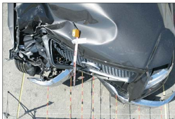
Figure 7: Top view of crush to front of case vehicle, baseline was set 10 cm (4 inches) beyond the vehicle's overall length to clear the displaced left bumper corner, each increment on rods is 5 cm (2 in)
