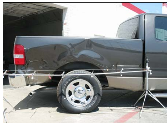
Figure 4: Damage to right side of case vehicle's truck bed from sideslap impact with left side of Chevrolet
