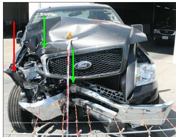
Figure 3: Damage to front of case vehicle from impact with the Chevrolet as well as the traffic signal pole (red arrow) and building (green arrows)
