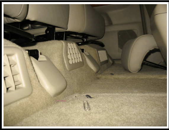
Figure 8. Location of the nickel metal-hydride batteries (under 2 nd row seats)
