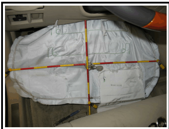
Figure 20. Driver's deployed knee air bag
