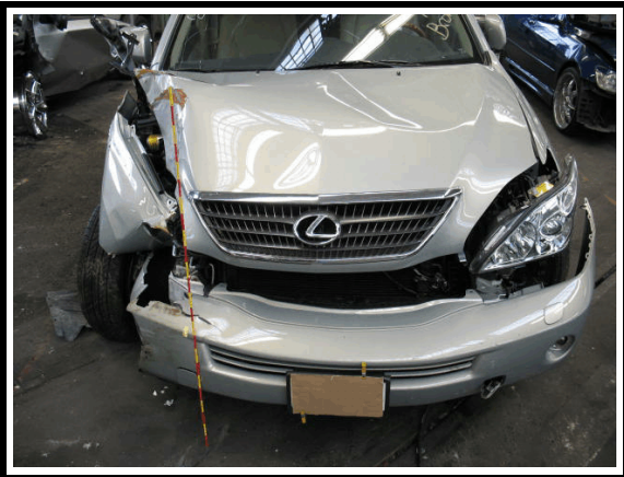
Figure 12. Front damage (bumper cover & right fender found inside vehicle)
