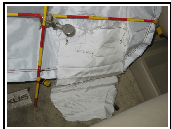
Figure 21. Additional piece of fabric stitched onto the lower right section of the knee air bag
