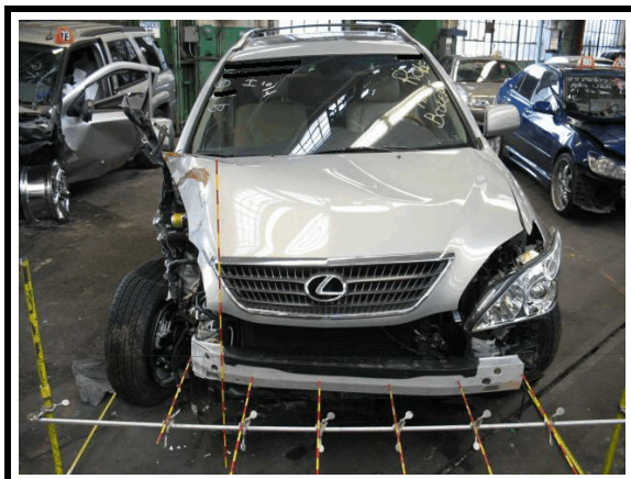
Figure 13. Front crush profile - 2006 Lexus RX440h
