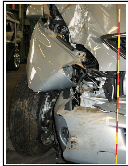
Figure 15. Close-up of direct damage from pole impact
