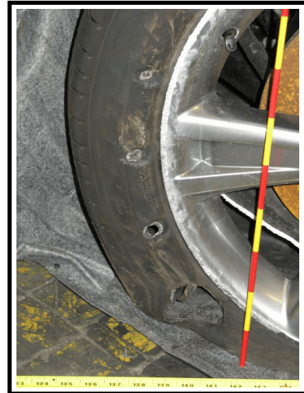
Figure 11. Closer view of holed/damaged RF tire sidewall
