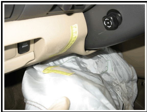
Figure 16. Deployed knee air bag and instrument panel scuff
