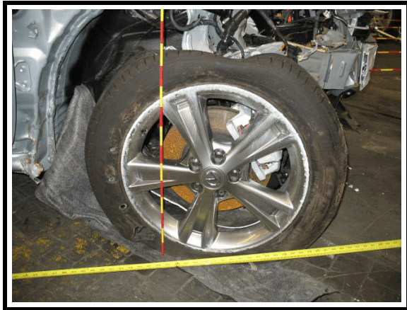
Figure 10. Damage to right front tire
