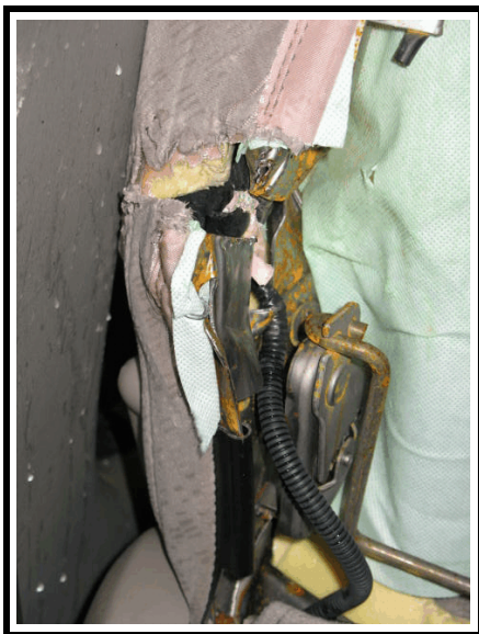
Figure 16. Driver's right seat back folding lock (cut by rescue personnel)
