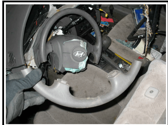
Figure 17. Bottom section of steering wheel cut off by rescue personnel
