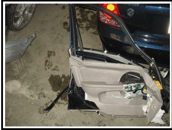
Figure 18. Left front door panel damage/intrusion (door cut off by rescue personnel)
