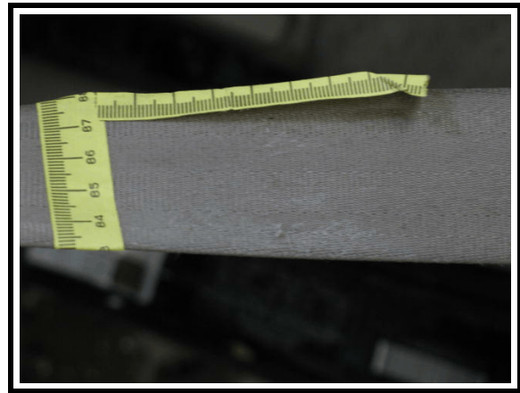
Figure 27. Close-up of occupant loading evidence on the driver's seat belt webbing
