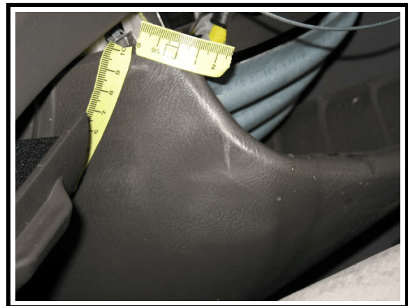
Figure 26. Occupant contact to lower steering column
