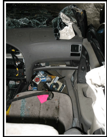
Figure 19. Intrusion/damage in RF seating area
