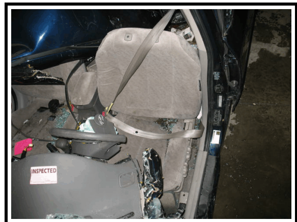
Figure 21. Driver's seat belt (evidence of occupant loading at the D-ring and near the latch plate)
