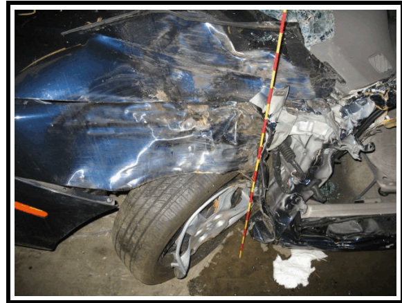
Figure 12. Left fender, hood and tire damage from the second tree impact
