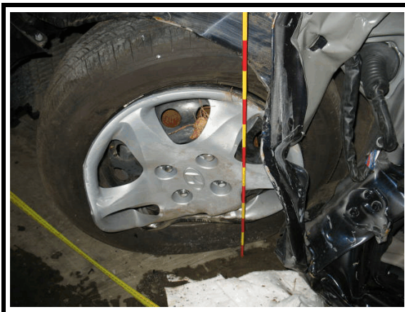
Figure 9. LF tire damage
