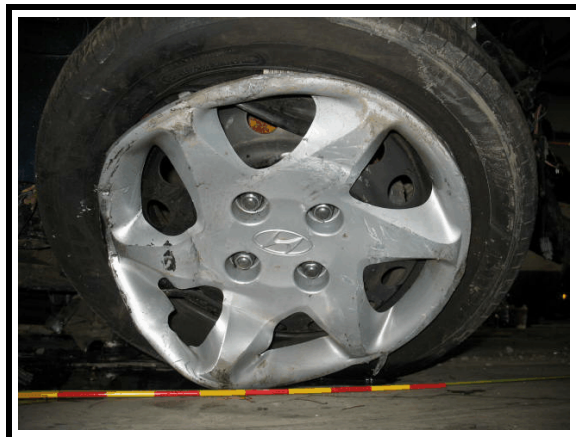
Figure 10. RF tire damage
