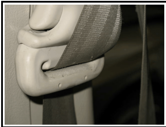
Figure 20. Evidence of occupant loading to driver's D-ring
