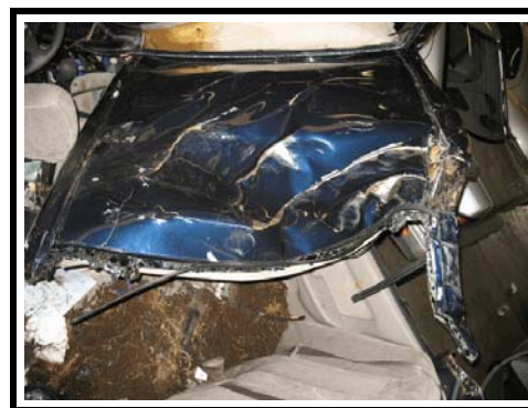
Figure 14. Roof damage (cut off by rescue personnel)
