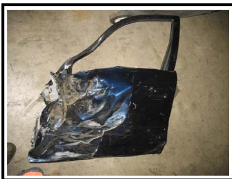
Figure 13. LF door damage (door cut off vehicle by rescue personnel)
