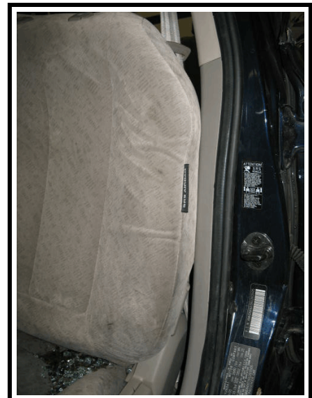
Figure 23. Location of the driver's seat back mounted side air bag (nondeployed)
