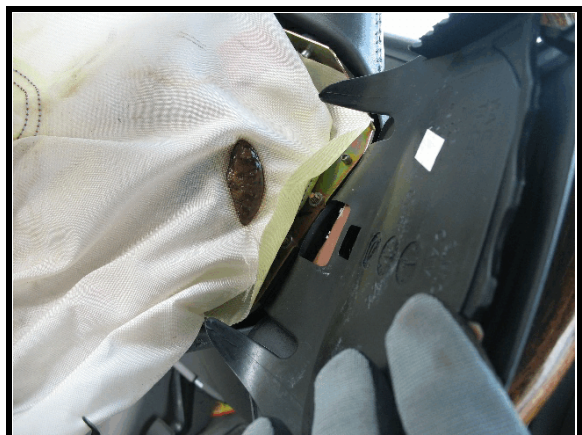
Figure 15. Melted plastic near inflator
