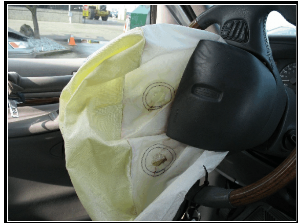
Figure 14. Driver's air bag, showing vent ports and top module cover
