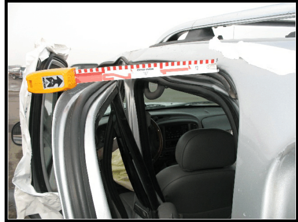
Figure 6. Gap at second row left door
