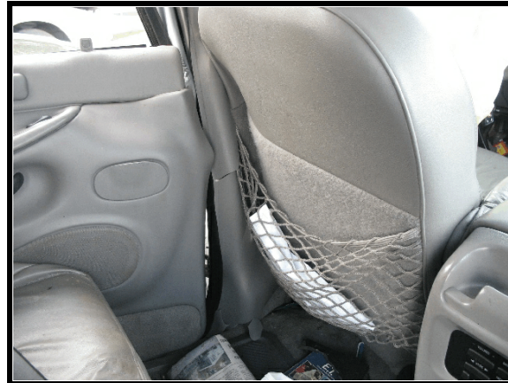
Figure 7. B pillar and left rear door intrusion
