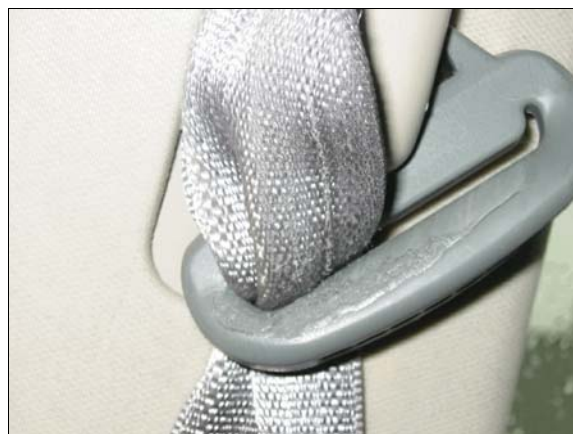
Figure 22: Front right passenger's shoulder belt jammed in front corner of "D"-ring and load marks on "D" ring
