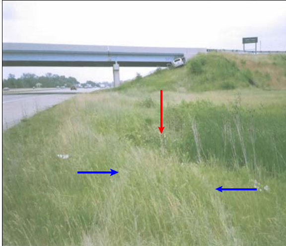
Figure 3: Police on-scene photo showing case vehicle approach to marshy area and impact with two small trees (red arrow), blue arrows show left and right side tire tracks in grass
