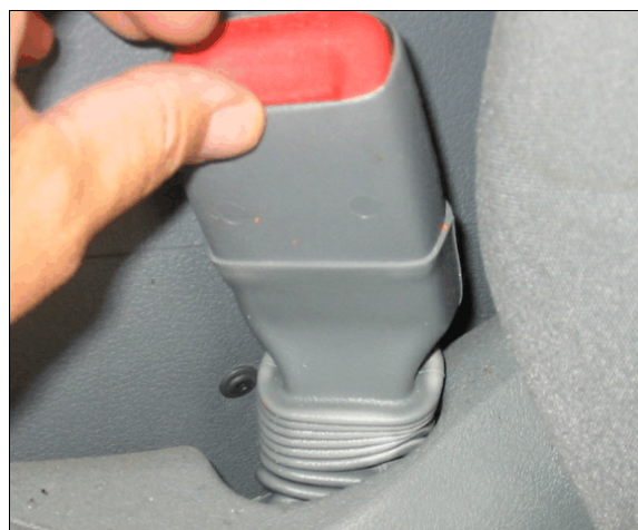
Figure 21: Driver’s buckle-mounted pretensioner actuated compressing the buckle stalk cover
