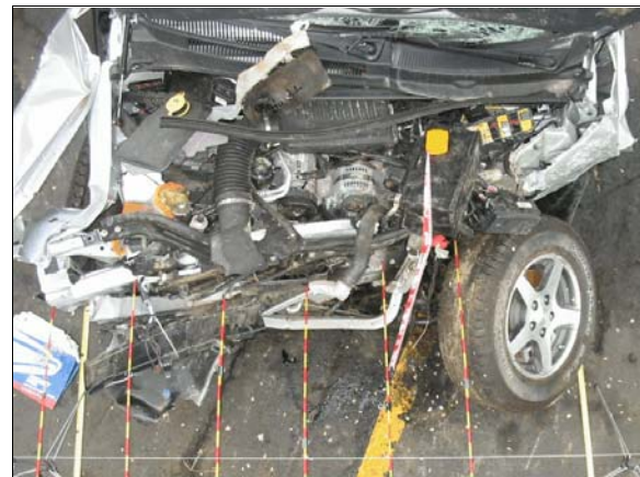
Figure 11: Top view of crush to front of case vehicle, each increment on rods is 5 cm (2 in)
