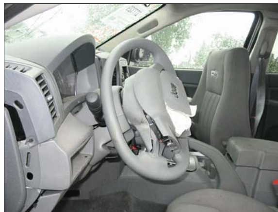
Figure 14: Left side view of damage to steering wheel and overview of forward displacement of front right seat back
