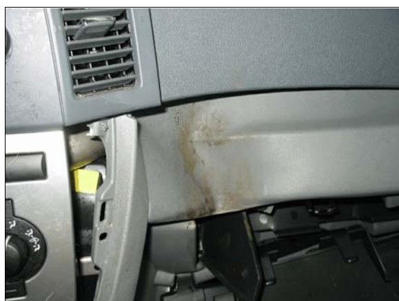
Figure 23: Dent in passenger knee bolster from impact by front right passenger’s left knee
