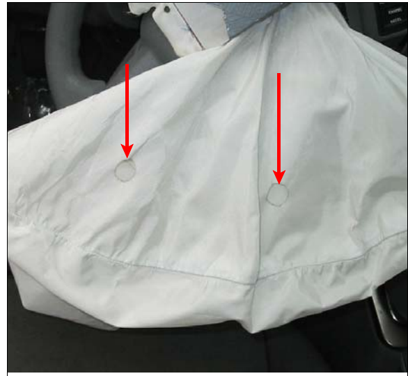
Figure 16: Case vehicle driver's air bag vent ports (arrows)
