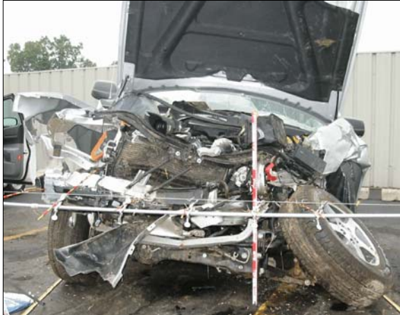
Figure 8: Damage to front of case vehicle primarily from impact with steel bridge deck support beam
