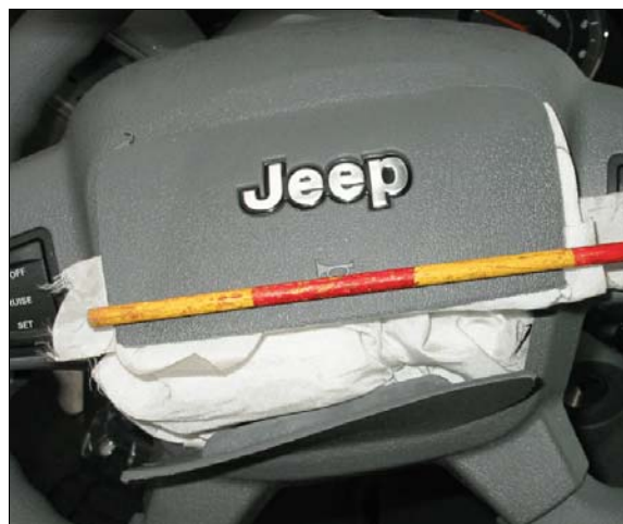
Figure 15: Case vehicle's driver air bag module cover flaps
