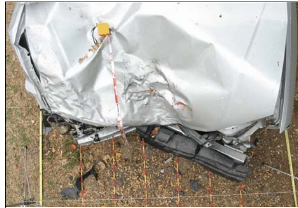
Figure 14: Top view of crush to front of Chevrolet from impact with the left side of the case vehicle
