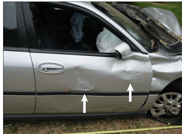
Figure 7: Damage to Chevrolet's right front door due to side-slap impact with case vehicle
