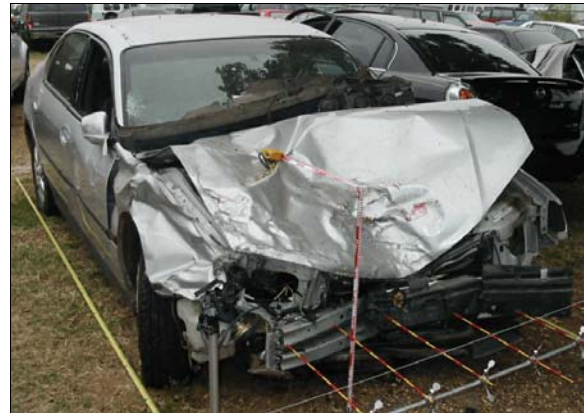
Figure 5: Overview of damage to front of Chevrolet from impact with left side of case vehicle
