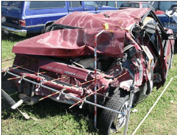
Figure 4: Damage to back of case vehicle from impact with Western Star, vertical scale in tenths of meter, each increment on rods is 5 cm (2 in)
