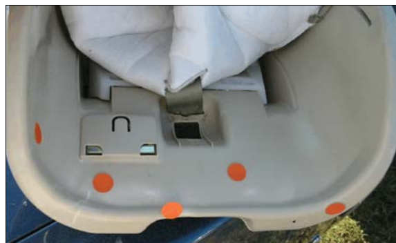
Figure 12: Orange dots show some of stress spots on the back left passenger's infant seat
