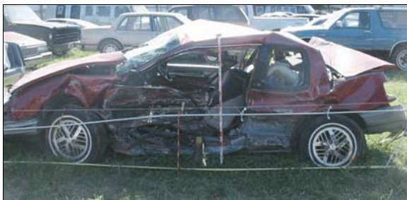
Figure 6: Damage to left side of case vehicle from impact with front of Chevrolet
