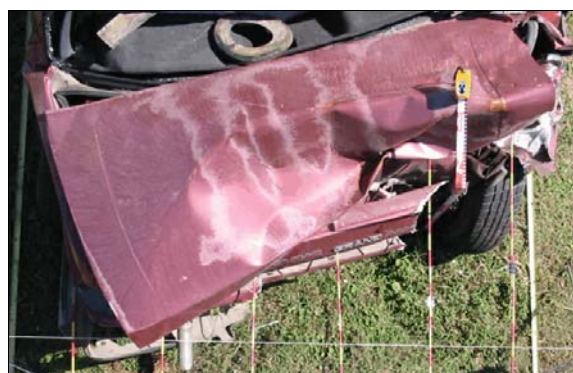
Figure 9: Top view of crush to back of case vehicle
