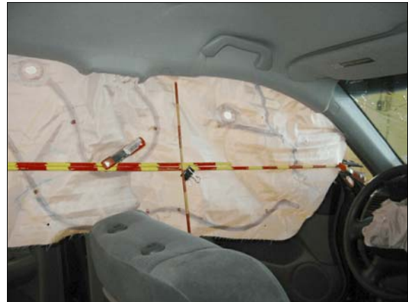
Figure 12: Overview of front portion of left side curtain air bag
