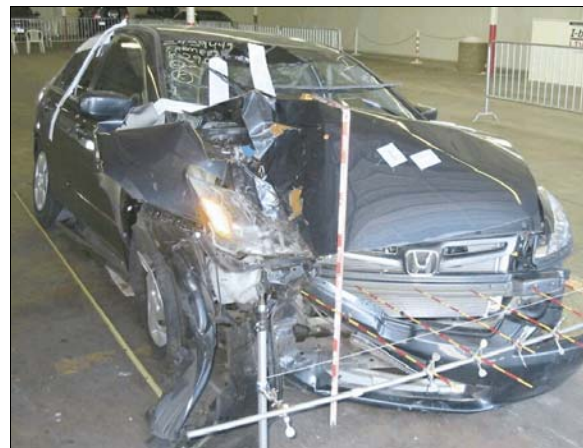
Figure 4: Overview of damage to front of case vehicle from impact with utility pole, vertical scale in tenths of meter, each increment on rods is 5 cm (2 in)
