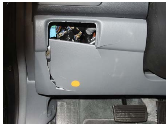
Figure 16: Damage to case vehicle driver's left knee bolster from driver's left knee impact
