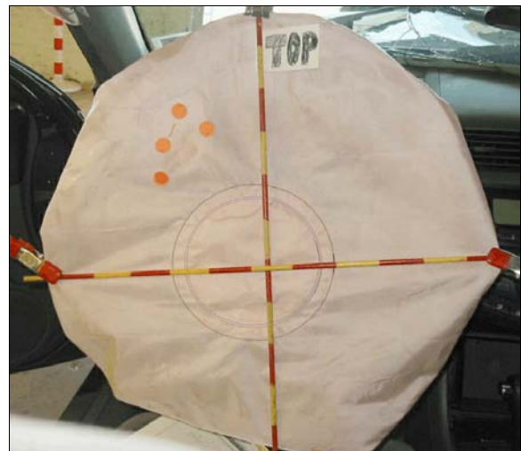
Figure 11: Case vehicle driver's air bag, orange dots show lip stick imprint
