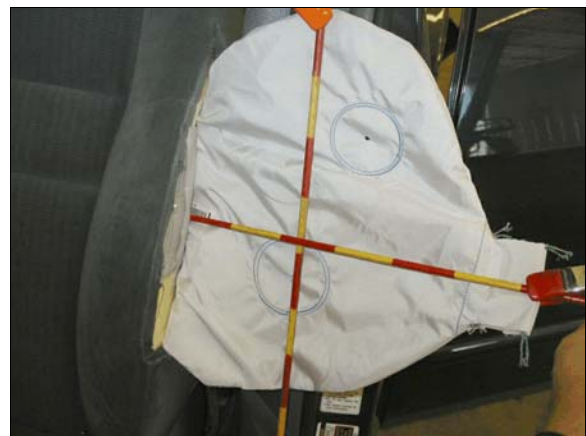
Figure 14: Inside surface of case vehicle driver's seat back-mounted side impact air bag
