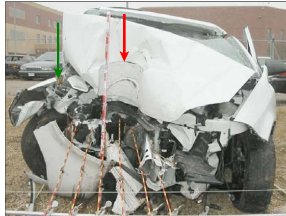
Figure 4: Damage to case vehicle from impact with clump of trees, red arrow shows impact location of tree that broke off, green arrow shows impact location of second tree, vertical scale in tenths of meter
