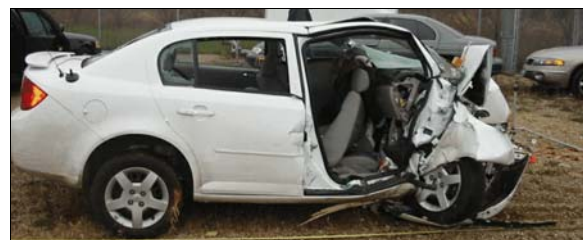
Figure 7: Right side view of crush to front of case vehicle from impact with clump of trees
