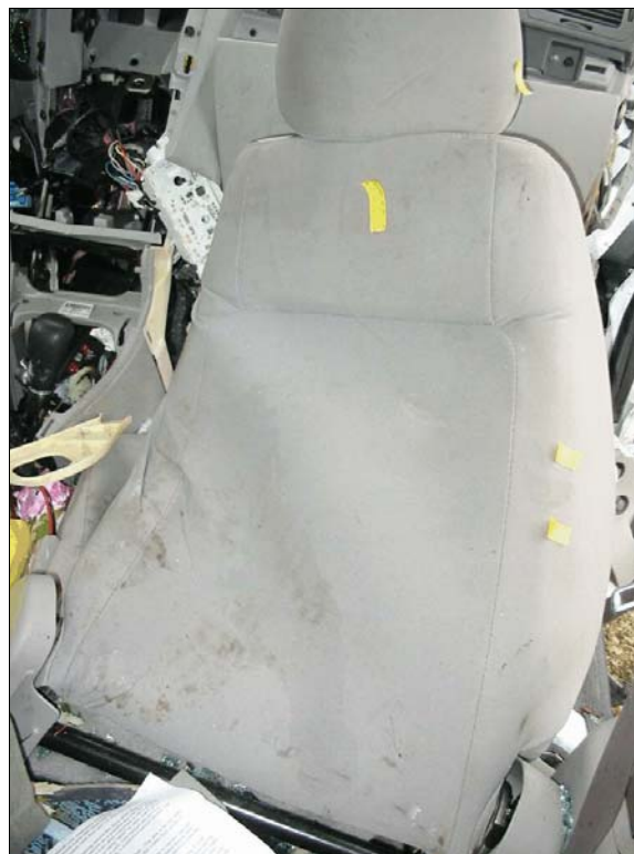
Figure 13: Damage to front right passenger’s seat back due to loading by unrestrained back right passenger
