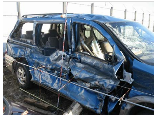
Figure 5: Damage to right side of case vehicle from impact by front of Freightliner, vertical scale increments in tenths of meter
