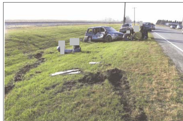
Figure 6: View southwest to case vehicle's rest position and tire furrows leading to rollover
