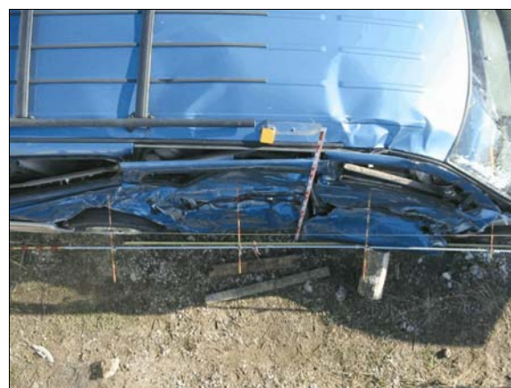
Figure 7: Top view of crush to right side of case vehicle’s passenger compartment due to Freightliner’s front impact, each increment on rods is 5 cm (2 in)
