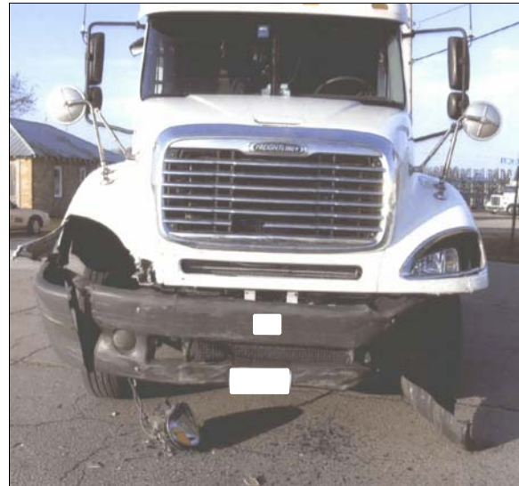
Figure 4: Sheriff department's on-scene photo of damage to front of Freightliner from impact with case vehicle
