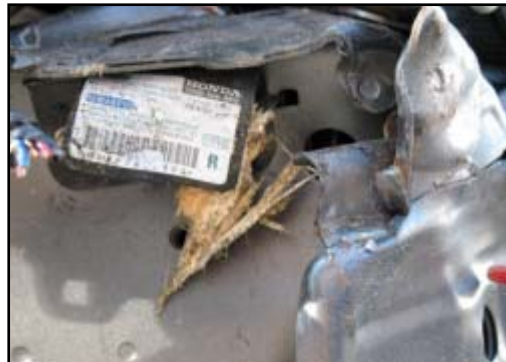
Figure 7. Damaged front right satellite air bag sensor.
