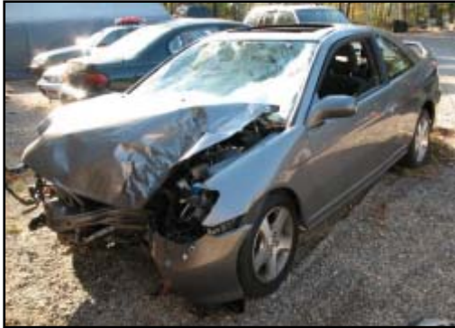
Figure 5. Residual frontal damage.
