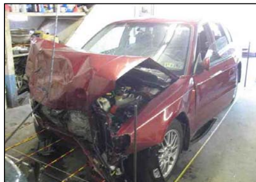
Figure 5 - Frontal damage to the Subaru Legacy.
