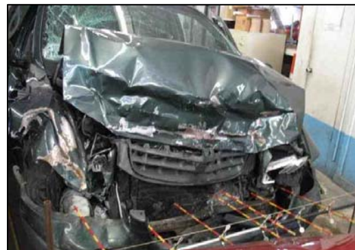
Figure 6 - Damaged frontal plane of the Chrysler Voyager.
