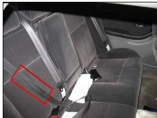
Figure 8 - Rear right lap and shoulder belt with potential loading evidence highlighted.
