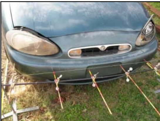
Figure 3. Resultant frontal damage and crush profile.
