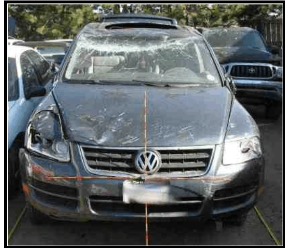
Figure 5. Overview of rollover damage
